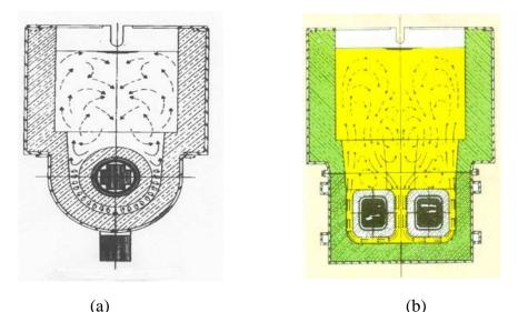
Figure 3: Circulation and metal flow (shown by the arrows) in a (3a) single loop inductor and (3b) double loop inductor.
