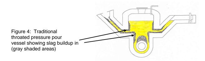
When sufficient buildup forms that prevents adequate heating of the metal, the inductor will have to be replaced because it can be extremely difficult to remove the buildup. Attempts to modify the furnace design with a throatless inductor (Figure 5) have been partially successful in eliminating buildup, but a periodic rigorous cleaning procedure is still necessary.
