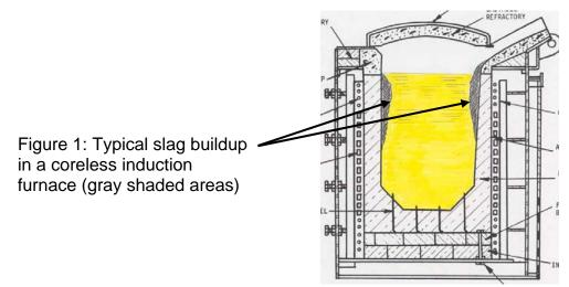
The hottest area of medium and high frequency coreless furnaces is at the mid-point of the power coil. All areas of slag deposit will be at a much lower temperature than those occurring at the center of the coil. Slag can also be deposited in areas midway down the crucible lining, where insufficient metal turbulence from magnetic stirring occurs.
