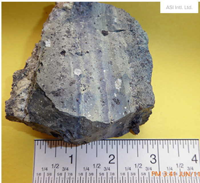
Figure 3. Insoluble buildup removed from Foundry G's coreless induction furnace after 48 hours of operation.
