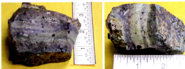
Figure 3: Removed slag build-up illustrating the progressive layering effect. ASI INTERNATIONAL
