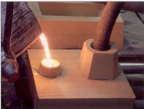
Fig. 3. Using a vacuum to assist in removing carbon laden decomposition products from the mold cavity improved the surface finish, though test castings still showed a very shiny, silvery surface with moderate deposits of lustrous carbon.
