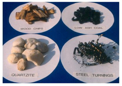
Figure 1: Ingredients used to make Ferrosilicon
