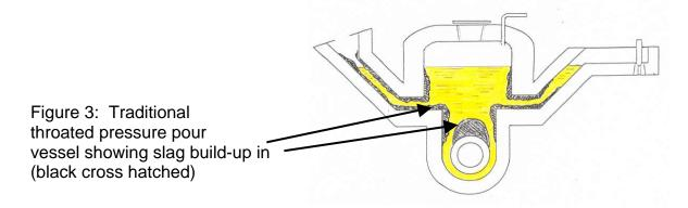
impossible, to remove the buildup. Attempts to modify the inductor with a throatless inductor (Figure 4) When this happens, the inductor will have to be replaced because it is extremely difficult, if not have been only partially successful in eliminating buildup.
