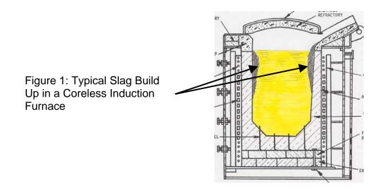
The areas of slag deposits are at a much lower temperature than the center of the furnace walls. Slag also is deposited in areas midway down the crucible lining, where insufficient metal turbulence from magnetic stirring occurs.
