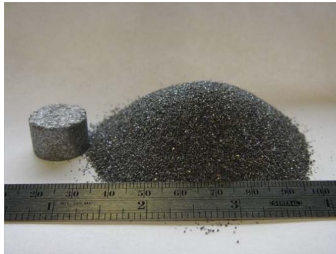
Fig. 12. Comparison of a 7.5 gram complex inoculant tablet to 75 grams of foundry-grade FeSi75, shown in a ratio of 1 to 10 reflecting the performance of 0.03% CAT to 0.3% FeSi75. CAT inoculant dimensions are 19 mm diameter and 11.6 mm high.
