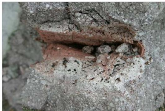
*Figure 8: Illustration of totally clogged inductor channel taken from a 10-ton channel furnace.*
