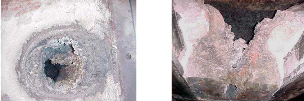
*Figure 3: Buildup in inductor channel (left) resulting in restricted metal flow and severely constricted throat opening, sectioned (right) illustrating heavy saturation.*
