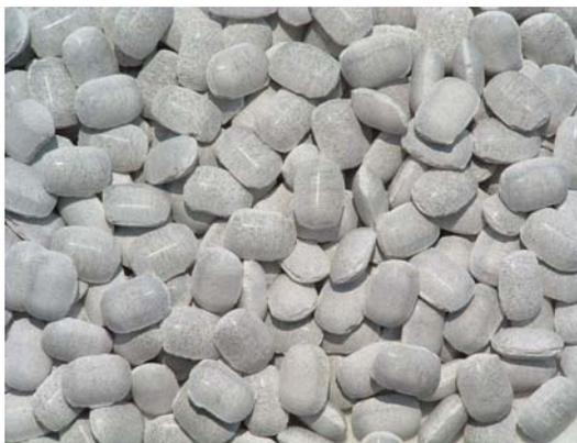
*Figure 7: Redux EF40L shown in briquetted form (14 gram tablets).*
