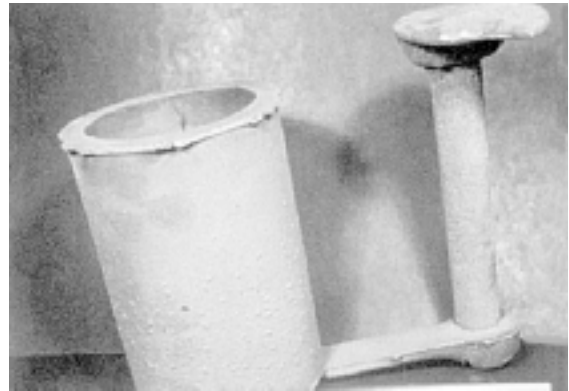
Fig. 2. Cylindrical test casting illustrating gating system used.
