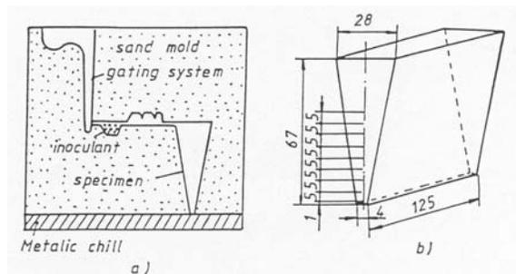
Figure 2. Schematic of a.) chill mold with in-mold chamber
