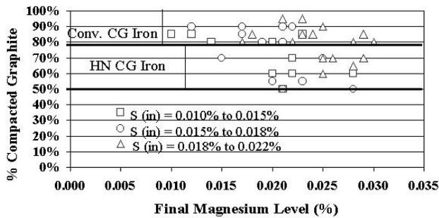
Figure 3: Influence of final residual magnesium  $Mg_{(fin)}$  on compacted graphite levels
