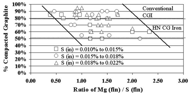
Figure 4: Influence of  $Mg_{(fin)}/S_{(fin)}$  ratio on the compacted on graphite level in the final iron structure
