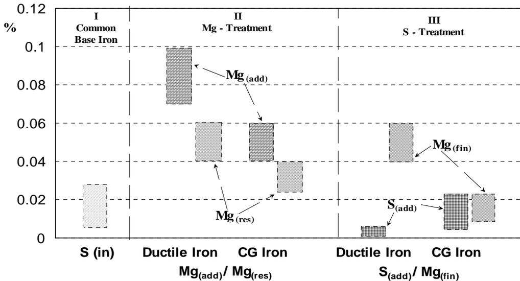
**Figure 1: CG Iron vs. Ductile Iron production from the same base iron by Mg-treatment and late S-addition with the post-inoculation**
