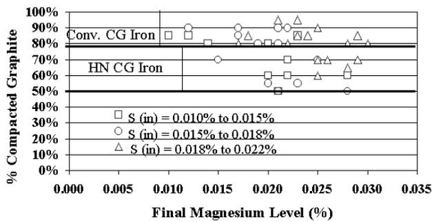
Figure 3: Influence of final residual magnesium  $Mg_{(fin)}$  on compacted graphite levels
