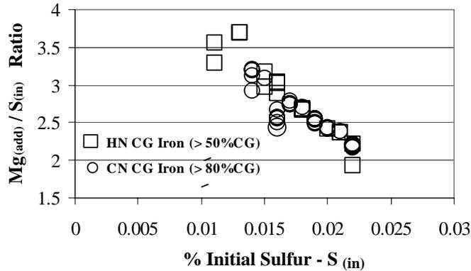
Figure 5: Effect of  $Mg_{(add)} / S_{(in)}$  ratio and on compacted graphite formation at varying initial sulfur ( $S_{(in)}$ ) levels
