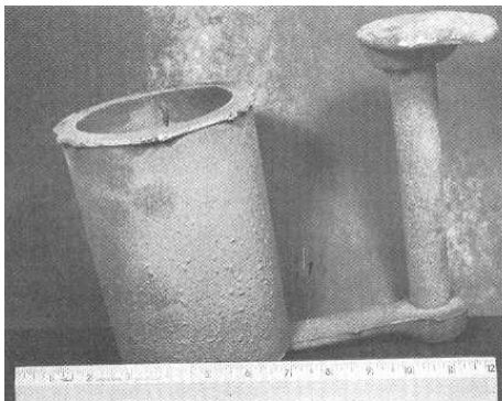
Figure 2: Cylindrical test casting illustrating gating system employed.
