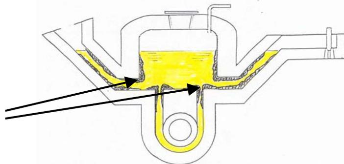
Depressurizing the pressure pour vessel and removing the top hatch for cleaning allows additional air to enter the vessel. This increases metal oxidation and worsens buildup problems. To remove the buildup for restoring electrical efficiency, it must be scraped from the side walls and inductor throats. If the buildup is hard, it is very difficult to remove. If the buildup is soft, then it is possible that
