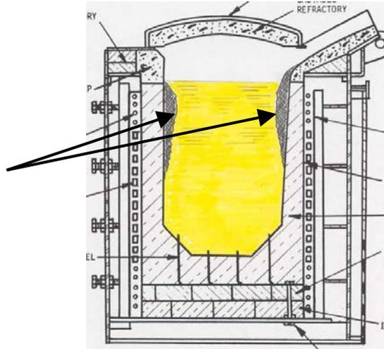
The areas of slag deposits are at a much lower temperature than the center of the furnace walls. Slag also is deposited in areas midway down the crucible lining, where insufficient metal turbulence from magnetic stirring occurs.
