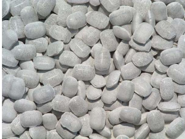
**Production Results:** To date, many foundries in the United States and Japan are using Redux EF40L sodium oxide-based fluxes to solve buildup problems in coreless induction furnaces, channel furnaces, pressure pour furnaces, Fisher converters, and ductile iron treatment ladles.
