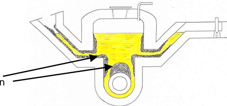
impossible, to remove the buildup. Attempts to modify the inductor with a throatless inductor (Figure 4) When this happens, the inductor will have to be replaced because it is extremely difficult, if not have been only partially successful in eliminating buildup.
