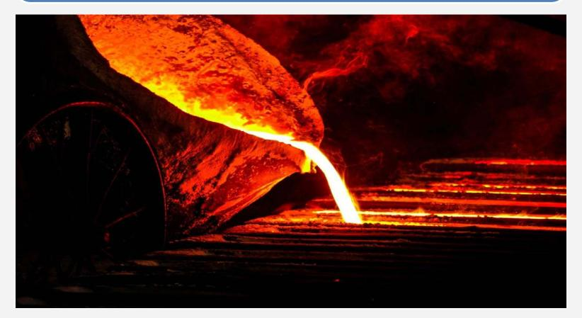
Field Trial of REDUX EF40L in a 1.5 Metric Ton Coreless Induction Furnace at International Foundry "M" pouring Grey and Ductile Iron
