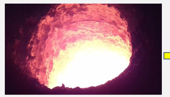
Lining condition after 1<sup>st</sup> Redux furnace addition
