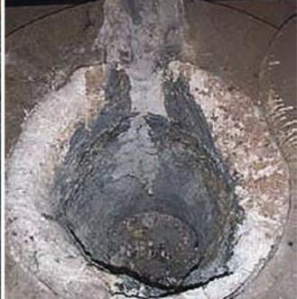
Evidence of the lining growth in the 500-lb. coreless induction furnace at Foundry X.
