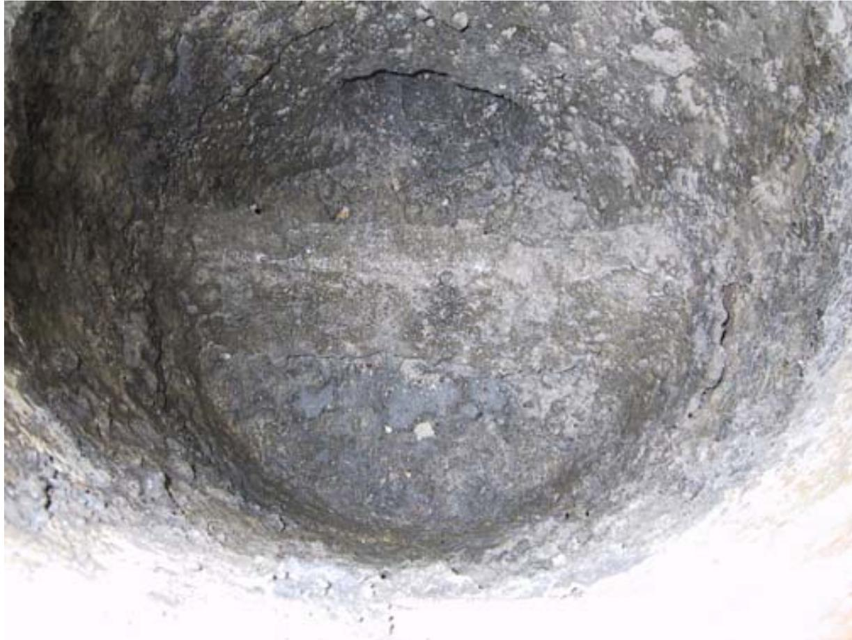
**Another overhead view focusing on the entrance of the pour spout into the ladle. Noted improvement in restoring the size of the opening.**
