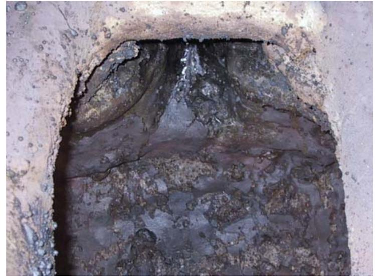
**Views of the spout of Ladle showing less restriction of the opening after the 5 wash treatments.**
