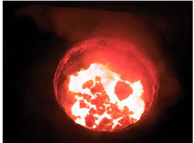
**Pictures illustrating the first and second addition of Redux EF40 L crushed briquettes for two consecutive wash heats. Note the turbulence on top of the bath.**
