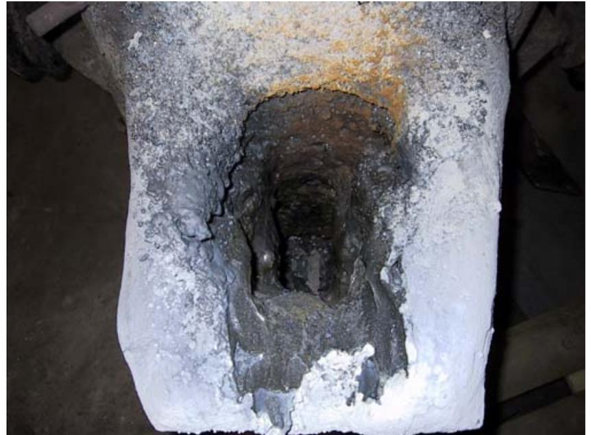
A Typical View of Ladle Slag after Treatment Process Has been completed. Also pictured is the pouring spout of the Ladle showing the build-up.
