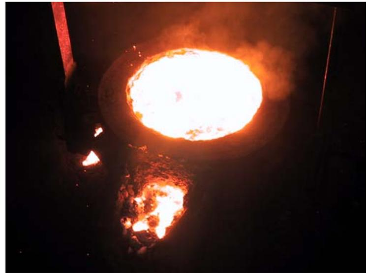
**Views of the Treatment Ladle being subjected to the third 1000Kg wash heat with 0.43 Kg Redux EF40L treatment.**
