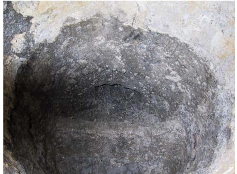
**Views of the second and third Redux EF40L flux treatments with individual wash heats. Each heat used 0.43 Kg(1lb) of Redux Flux per 1000Kg of Molten Iron. A noticeable improvement in cleanliness of the refractory sidewall and treatment pocket.**
