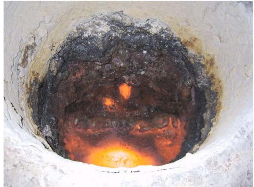
**Views of the fourth wash heat treatment with 0.43Kg Treatment of Redux EF40L. Note the vigorous reaction with the slag. The Gas being released is carbon dioxide, NO Fluorine or Chlorine**
