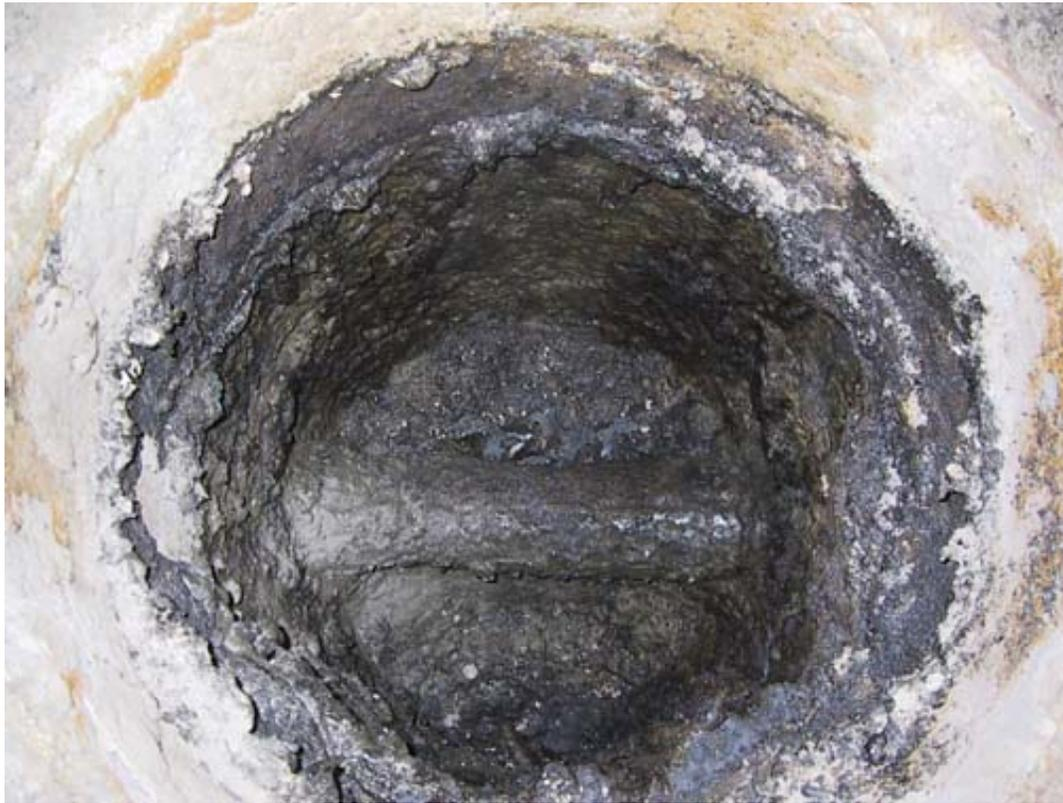
**An overhead view of the ladle after the 5 wash heats in a cold state. Noticeable definition of the pocket was evident.**
