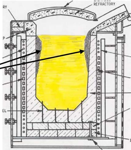
The hottest area of medium and high frequency coreless furnaces is at the mid-point of the power coil. All areas of slag deposit will be at a much lower temperature than those occurring at the center of the coil. Slag can also be deposited in areas midway down the crucible lining, where insufficient metal turbulence from magnetic stirring occurs.
