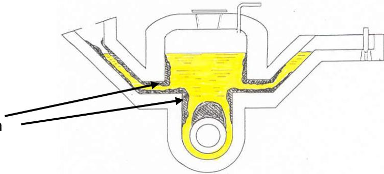
When sufficient buildup forms that prevents adequate heating of the metal, the inductor will have to be replaced because it can be extremely difficult to remove the buildup. Attempts to modify the furnace design with a throatless inductor (Figure 5) have been partially successful in eliminating buildup, but a periodic rigorous cleaning procedure is still necessary.
