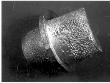
*Figure 3: Surface pockmarking on steel casting*
