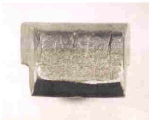
*d: Surface wrinkles on pulley hub*
