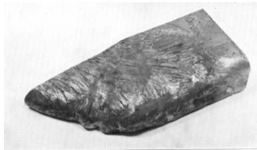
*Figure 7: Severe surface wrinkling resulting from solidification against accumulations of lustrous carbon*
