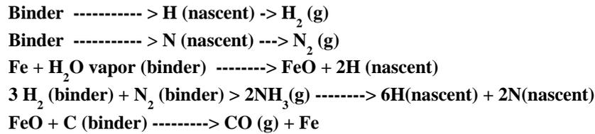
Although the first four reactions are likely to promote both surface and subsurface porosity defects, the last reaction usually results only in surface defects, such as surface pockmarking or, more frequently, lustrous carbon laps and surface wrinkles (Naro 1977).
