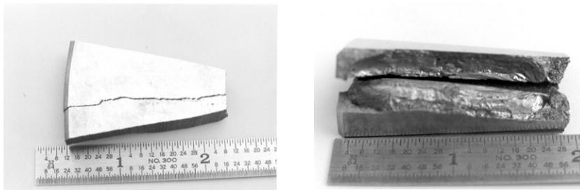
**a. Top view of braking surface with defect**
