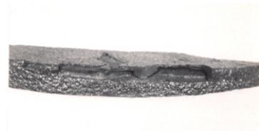
*c: Surface lamination on disc brake*
