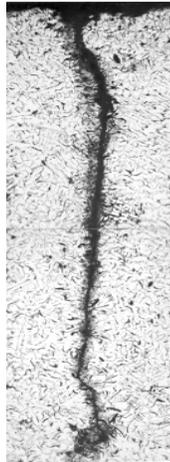
**Figure 14: Microstructure of casting containing severe lustrous carbon “leaker” in gray iron,**
