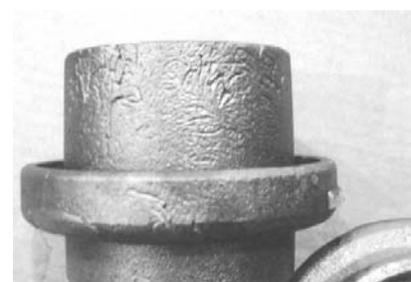
*f: Surface wrinkling on lost foam truck transmission part*
