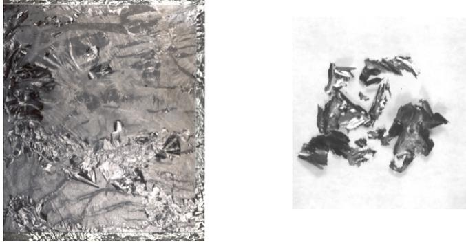
*Figure 5: Examples of lustrous carbon films adhering to test casting at shakeout*
