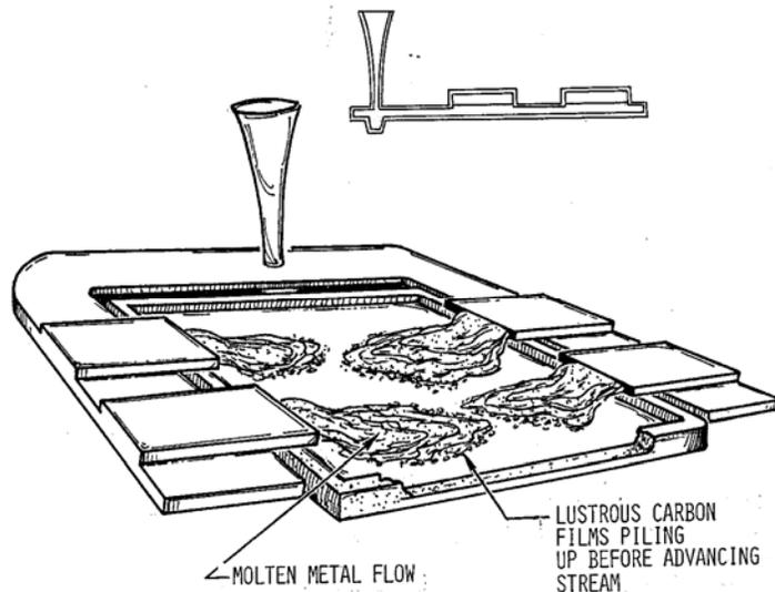
**Figure 12: Metal flow pattern in test casting**
