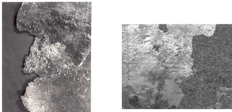
*Figure 8: Layer of lustrous carbon bonded sand (left) and cast surface from which bonded layer was removed (right)*
