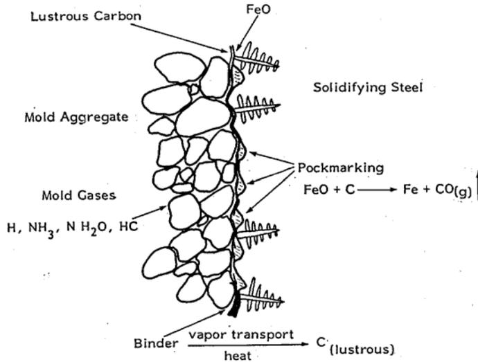
**Figure 16: Proposed mechanism of pock making or surface porosity resulting from lustrous carbon reactions in steel**
