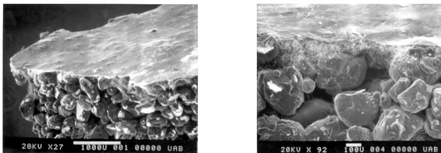
*Figure 11: SEM Photographs showing a continuous carbon layer attached to the mold surface after metal pouring*
