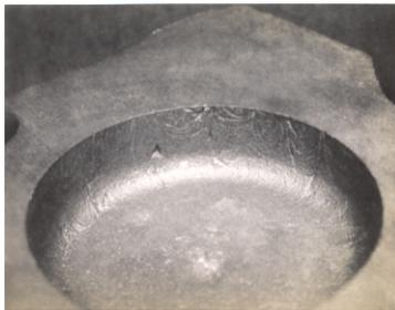
*a: Wrinkles on automotive brake caliper*
