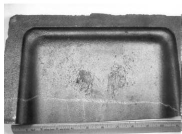
*e: Surface wrinkles in oil pan which leaked*
