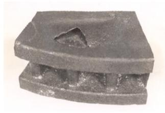
*b: Blister on disc brake rotor*
