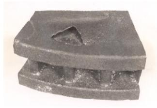
*b: Blister on disc brake rotor*
