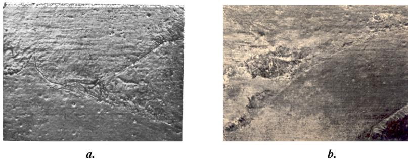
**Figure 13: Examples of severe surface wrinkling from lustrous carbon formation in test castings**
