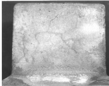
*Figure 10: Scab-block castings made with premium quality furan no-bake binder, no iron oxide*
