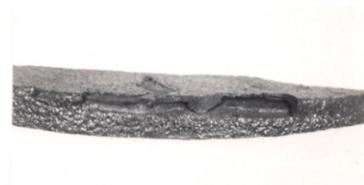
*c: Surface lamination on disc brake*
