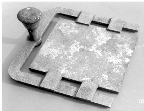
*Figure 4: Configuration of lustrous carbon test casting, 9 inches long by 8 inches wide by ½ in thick, sprue choke – ½ inches*
