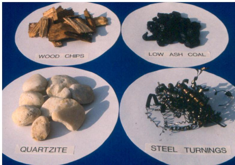
Figure 1: Ingredients used to make Ferrosilicon
