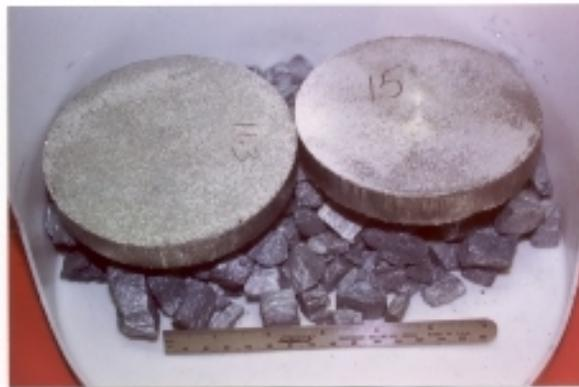
Figure 8. Illustrations of Nodu-Disc iron magnesium nodulizing discs covering magnesium ferrosilicon. Magnification 0.5x
