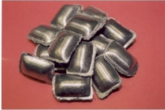
Figure 7. Photograph of Nodu-Bloc iron-magnesium briquettes magnification 1.25x
