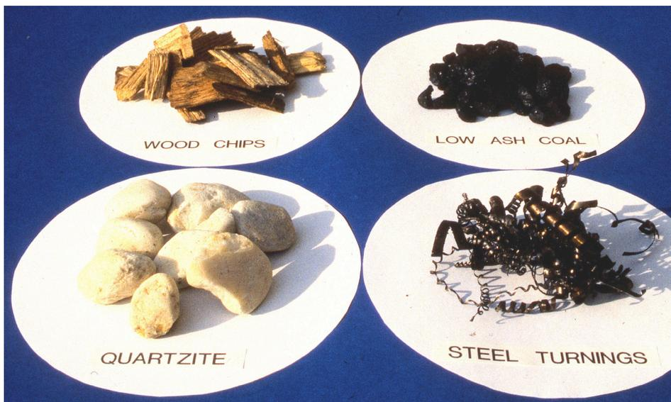
**Figure 1.** Ingredients used to make Ferrosilicon
